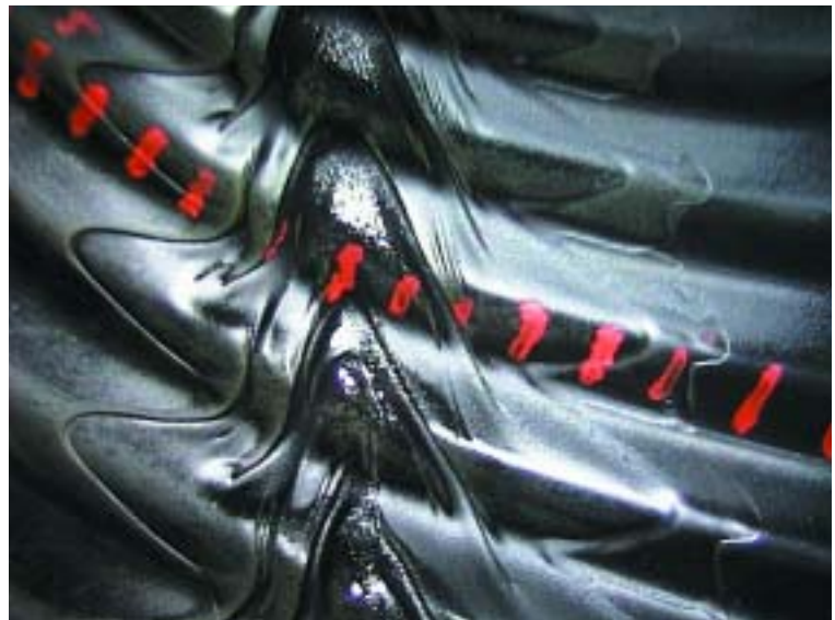
FIGURE 9. Polymer modified asphalt paved invert over Polymer Precoat after Test run 8.
