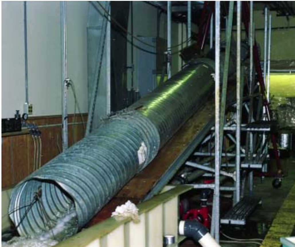
FIGURE 1A. Accelerated Abrasion Test Apparatus.
