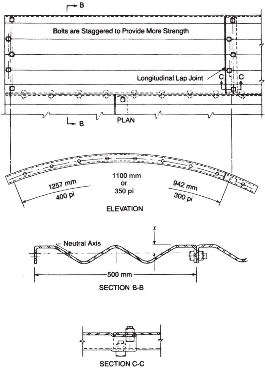
Figure 11.2 Details of 2-flange liner plate.
