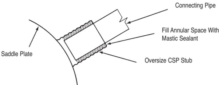
**Figure 2.23** Universal connection detail using saddle branch.
