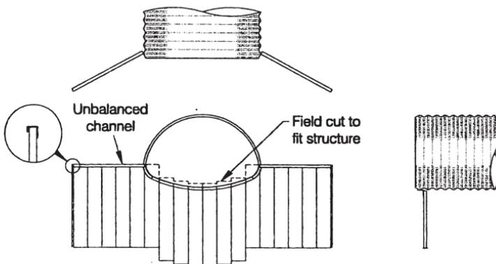
**Figure 2.26** Illustration of how a steel sheeting headwall can be provided for a pipe-arch culvert.
