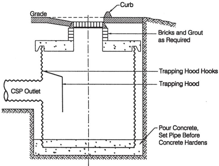
**Figure 2.25** Cross sections of catch basins.
