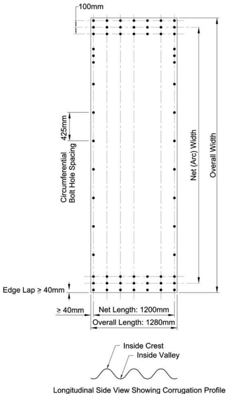
**Figure 2.15** Deep Corrugated Structural Plate Type II plate configuration
