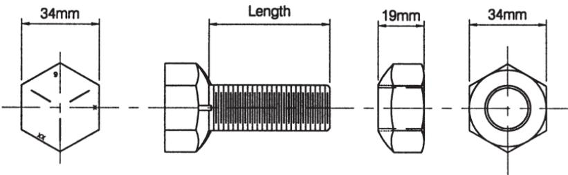
**Figure 2.8:** Dimensions of bolts and nuts for structural plate.
