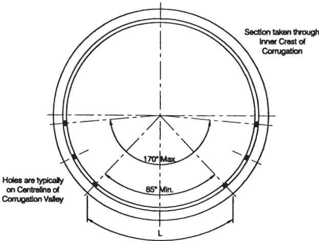
**Figure 2.2** Invert perforating detail.
