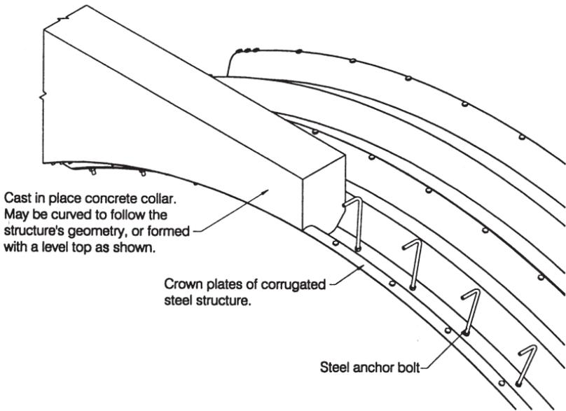
Figure 2.33 Concrete end reinforcing collar.
