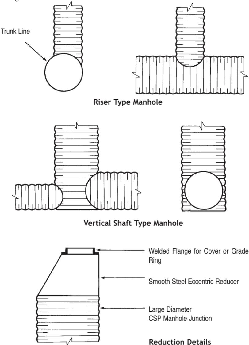
**Figure 2.24** Illustration of types of CSP manholes.
