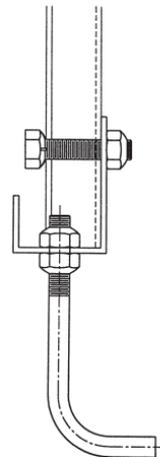
**Figure 2.10:** Hook bolt and base channel.
