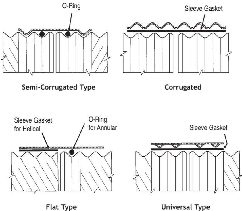
**Figure 2.18** Standard CSP band types. Note: When gaskets are required they are installed with standard CSP band types as shown.
