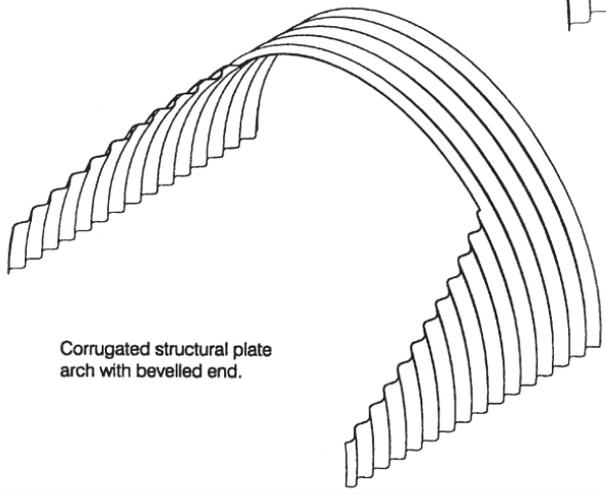
Corrugated structural plate arch with bevelled end.
