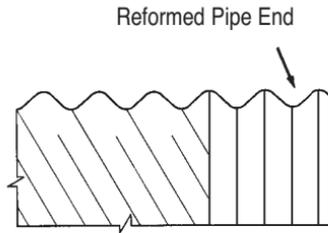
**Figure 2.17** Reformed end of helically corrugated pipe.
