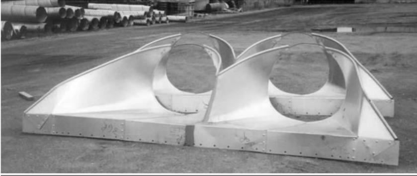
Special fabricated twin end sections.
