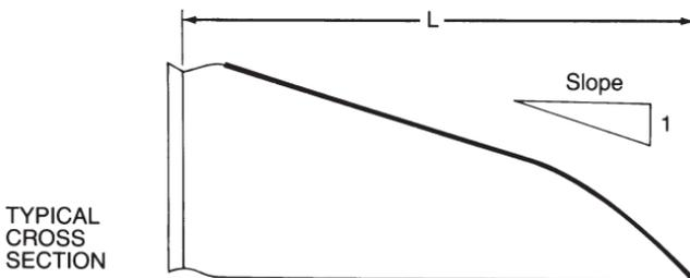
Figure 2.27 Details of end sections in round and pipe-arch shapes.
