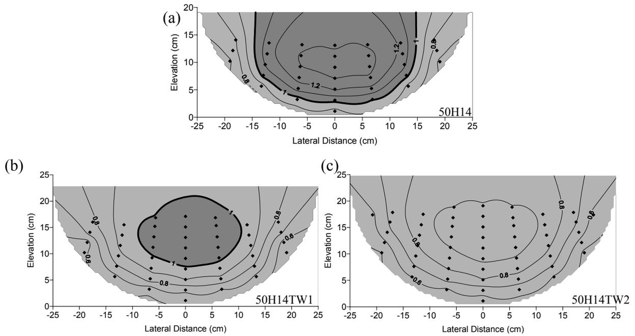
Figure 5. Distribution of  $V_x$  non-dimensionalized with respect to  $V_{\text{mean}}$  at hole 14 for a discharge of 50 L/s and: (a) tailwater depth set at normal depth, (b) tailwater depth set at 4.4 cm above normal depth, and (c) tailwater set at 6.4 cm above normal depth.
