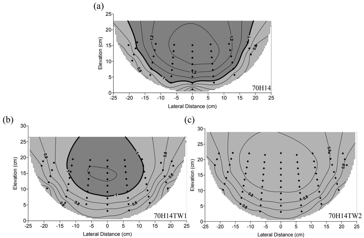
Figure 6. Distribution of  $V_x$  non-dimensionalized with respect to  $V_{\text{mean}}$  at hole 14 for a discharge of 70 L/s and: (a) tailwater depth set at normal depth, (b) tailwater depth set at 4.4 cm above normal depth, and (c) tailwater set at 6.4 cm above normal depth.
