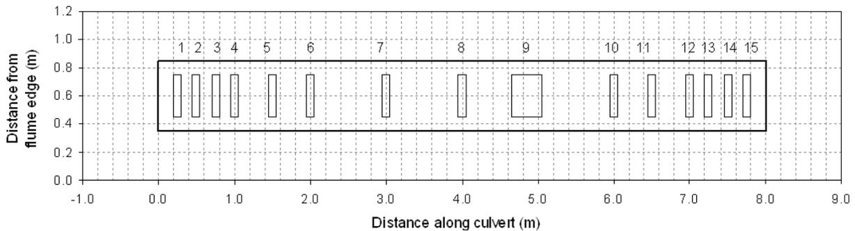
Figure 1. Plan view of culvert showing location and size of culvert access holes.
