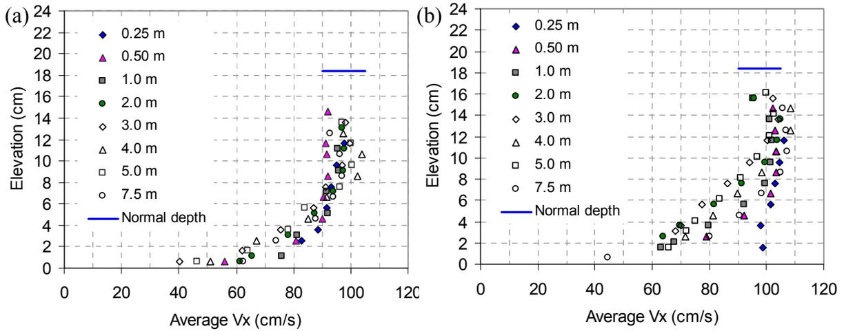
Figure 4. Centerline vertical velocity profiles for (a) 50 L/s and (b) 70 L/s.
