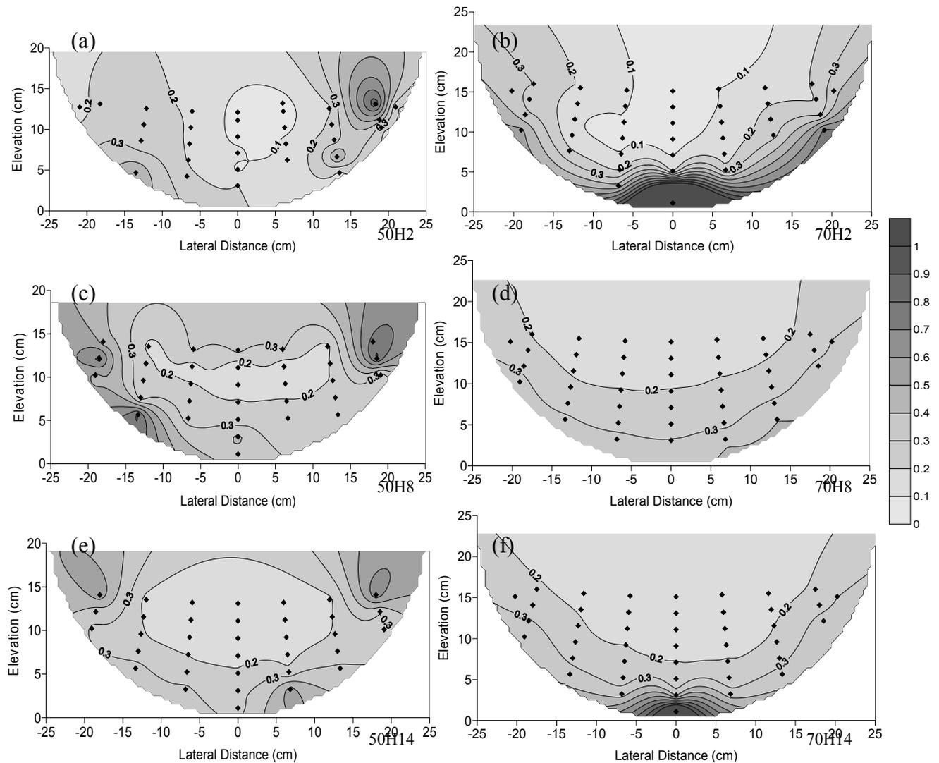
Figure 7. Distribution of  $I_{mag}$  for (a) 50 L/s at hole 2, (b) 70 L/s at hole 2, (c) 50 L/s at hole 8, (d) 70 L/s at hole 8, (e) 50 L/s at hole 14, and (f) 70 L/s at hole 14.
