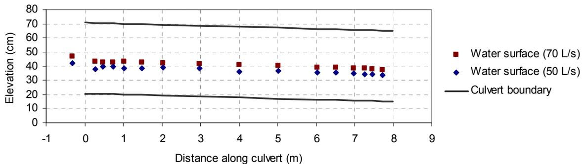
Figure 3. Water surface profiles for discharges of 50 L/s and 70 L/s.
