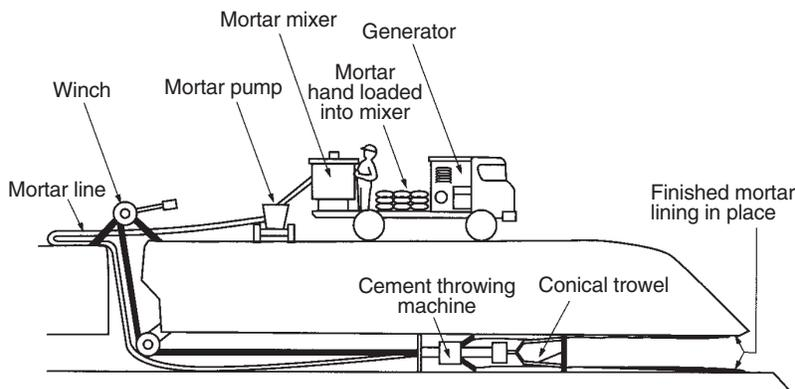
Figure 11.5 Cement Mortar Lining
